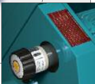
Speed control and speed chart on variable speed model KC1016VS
