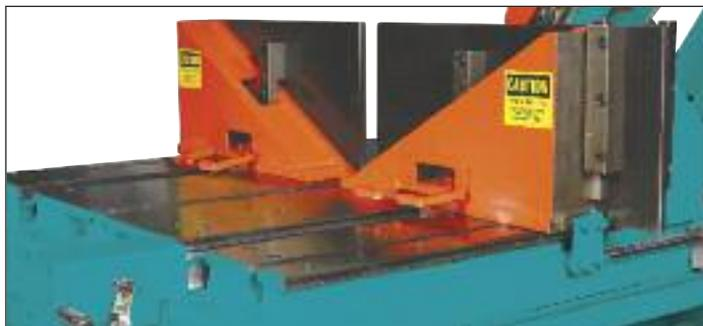
Hydraulic Rack Gear Vice (**standard on model VG450MP**) is operated from the control panel. Independent operation of the left and right jaw or both jaws together.
