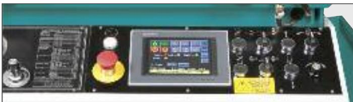
Front mounted control panel that controls all sawing functions such as saw frame tilt, blade speed, saw frame cant, right & left vise clamp/release, guide arm up/down, easy to read blade speed chart and a HMI touch screen.
