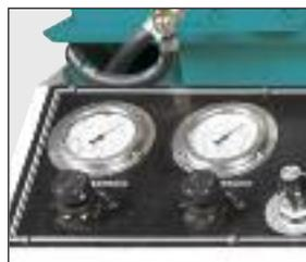
Hydraulic pressure gauges are mounted in the control panel. This lets the operator to easily adjust the blade cutting pressure and on models equipped with a hydraulic vise will let the operator adjust hydraulic vise grip pressure.
